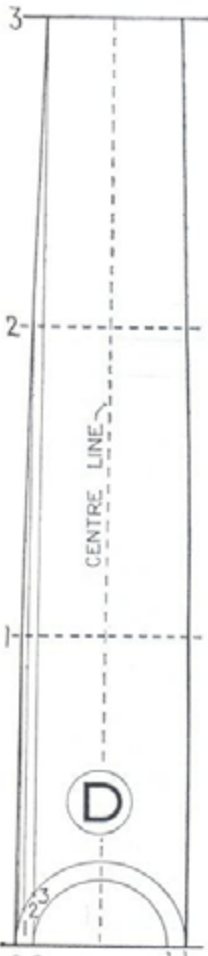
D METHOD FOR ENTASIS abc d ARE BOTTOM & TOP DIAMETERS RESPECTIVELY. DESCRIBE SEMICIRCLES ON THESE & AT c ERECT PERPENDICULAR CUTTING LARGER ONE IN 3. DIVIDE SEGMENT a 3 & HEIGHT OF COLUMN INTO ANY NUMBER OF EQUAL PARTS - SAY 3 - & NUMBER BOTH 1,2,3 FROM a. THRO' POINTS 1,2,3 IN SEGMENT ERECT PERPENDICULARS CUTTING CORRESPONDING DIVISIONS OF THE HEIGHT. THRO' THE POINTS THUS OBTAINED DRAW CURVE
